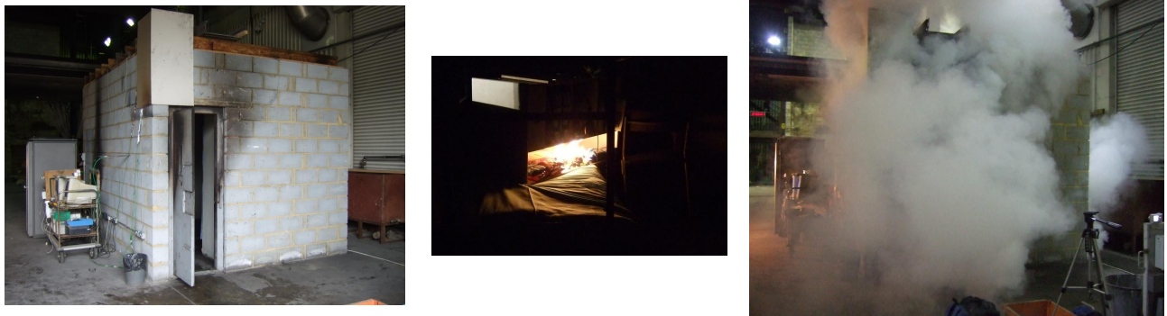
Figure 9 – Photographs showing test room, fire scenario and aerosol discharge shortly after activation
